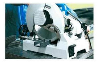
Exhibit 3 depicts a Makita Cold Cut-Off Saw with Serrated Cutting Teeth (1.75 kW input power).
